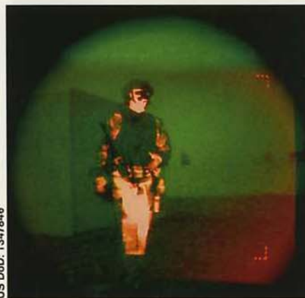
■ ITT's ENVG system, soon to be developed into a digital sensor, provides operators with not only infrared capability but also thermal imaging for increased detection in built-up areas.
