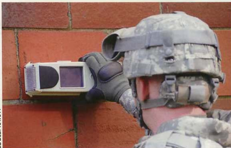
■ Sense Through Wall sensors will soon be fielded to US forces in order to improve situational awareness before entering buildings and compounds.
