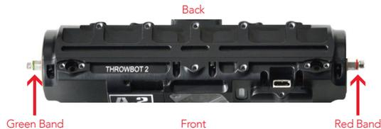
5. Replace the hex nuts using the 5/16" nut driver.
